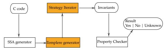
The shaded modules are modified to make 2ls handle the array segmentation.
