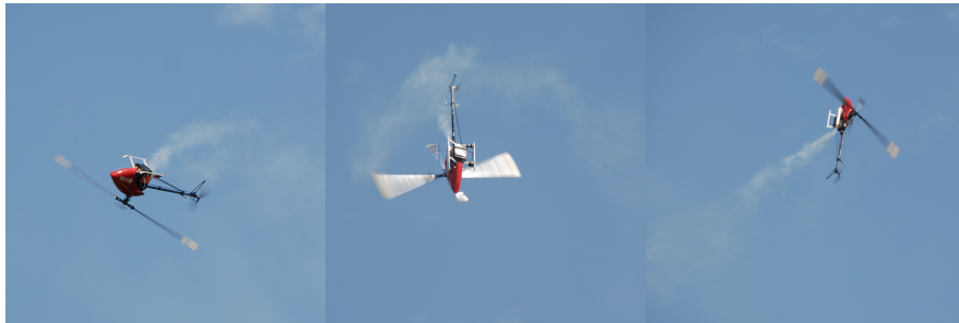
Figure 1: The dynamical modeling method presented in this work is used to model a helicopter’s dynamics as it is flown through aerobatics. A unified model is learned for a rich array of maneuvers, including flips, loops, stop and go, vertical sweeps, circles, dodging, orientation sweeps, gentle freestyle, tictocs, chaos, and aggressive freestyle.
