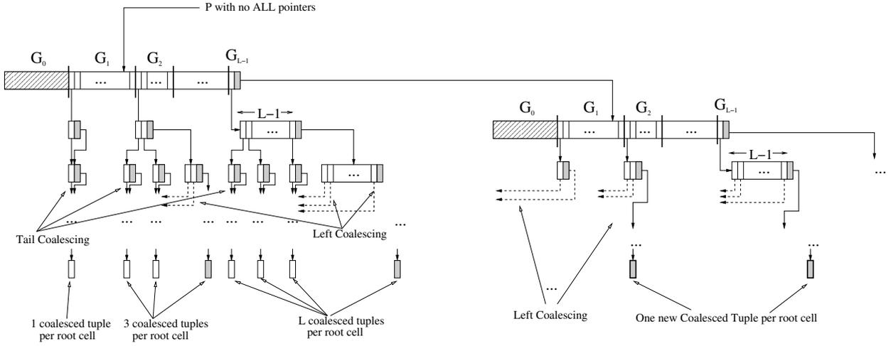
Figure 8: Tail-Coalesced partitioned node with  $T = C$
