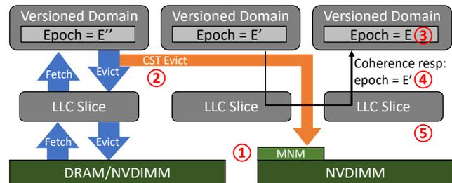
Fig. 1: **NVOverlay Features** – ① – Multi-snapshot NVM Mapping (MNM); ② – Coherent Snapshot Tracking (CST) and background persistence; ③ – Distributed epochs; ④ – Coherence-driven epoch synchronization; ⑤ – Distributed LLC support.
