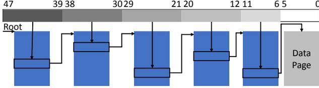
Fig. 10: **Master Mapping Table** – Shows five-level radix tree structure. Blue represents index pages while grey represents data.
