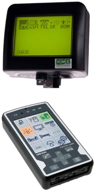
Figure 1. HMC "Easy Rider" (top) and "Gewa Control Omni" (bottom), two multifunctional interfaces for people with disabilities, operated through switches or scanning.
