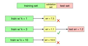
• The test set is used only at the very end, to measure the generalization performance of the final configuration.
