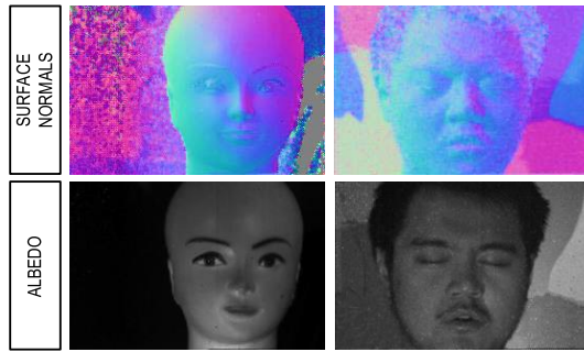
Fig. 14. Experimentally measured single-frame photometric stereo imaging results: surface normals maps and albedo maps generated at 20 frames/s, for both static (left) and dynamic (right) scenes [14].
