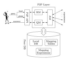
Figure 3: Architecture for a PDBMS
