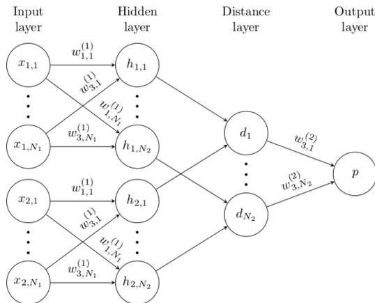
Figure 3. A simple 2 hidden layer siamese network for binary classification with logistic prediction  $p$ . The structure of the network is replicated across the top and bottom sections to form twin networks, with shared weight matrices at each layer.
