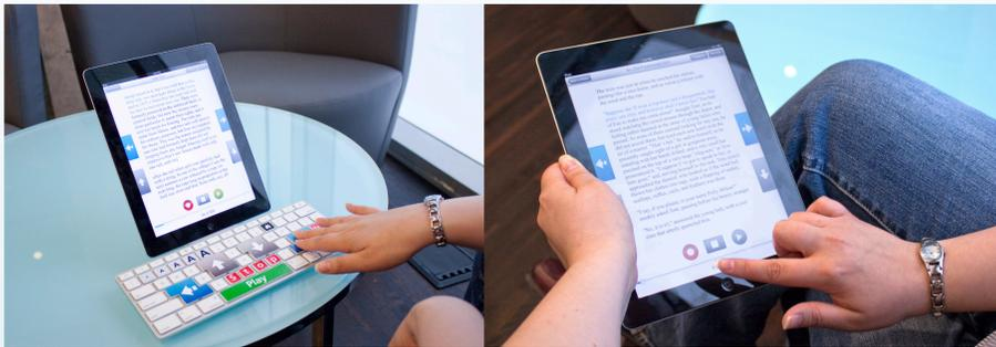
Alongside standard touch screen gestures, the ALLT book can be controlled using a wired or wireless keyboard with large target buttons. An exploration into voice commands is currently underway.
