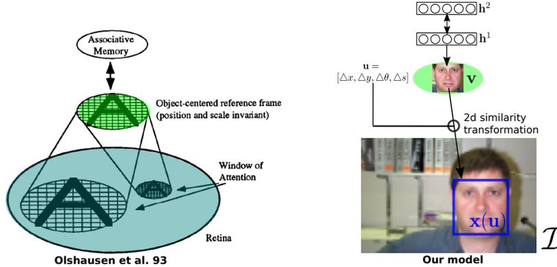
Figure 1: **Left:** The Shifter Circuit, a well-known neuroscience model for visual attention [13]; **Right:** The proposed model uses 2D similarity transformations from geometry and a Gaussian DBN to model canonical face images. Associative memory corresponds to the DBN, object-centered frame correspond to the visible layer and the attentional mechanism is modeled by 2D similarity transformations.
