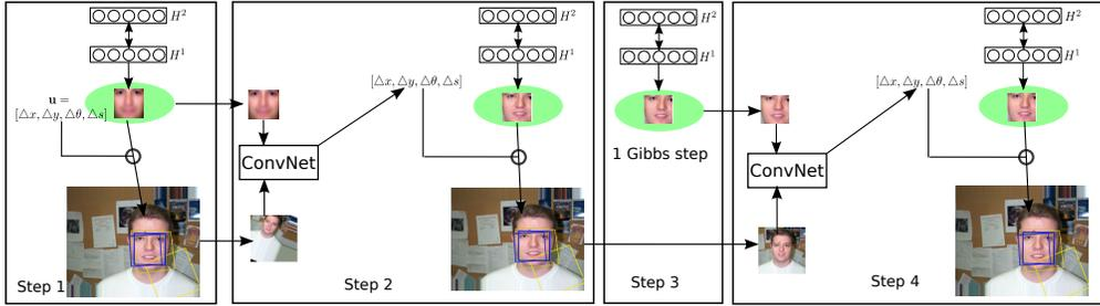
Figure 3: Inference process:  $\mathbf{u}$  in step 1 is randomly initialized. The average  $\mathbf{v}$  and the extracted  $\mathbf{x}(\mathbf{u})$  form the input to a ConvNet for approximate inference, giving a new  $\mathbf{u}$ . The new  $\mathbf{u}$  is used to sample  $p(\mathbf{v}|\mathcal{I}, \mathbf{u}, \mathbf{h})$ . In step 3, one step of Gibbs sampling of the GDBN is performed. Step 4 repeats the approximate inference using the updated  $\mathbf{v}$  and  $\mathbf{x}(\mathbf{u})$ .
