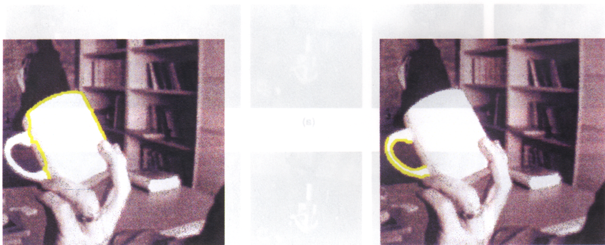
Fig. 5. Aspect-based object recognition by parts. The cup is composed of two parts, the handle and the body. Although the cup grasp and pose are perhaps not those usually encountered in day-to-day use, the example is illustrative of the recognition process. The parts must be visible in an image in order to be recognized and this is possible in a wide variety of poses.
