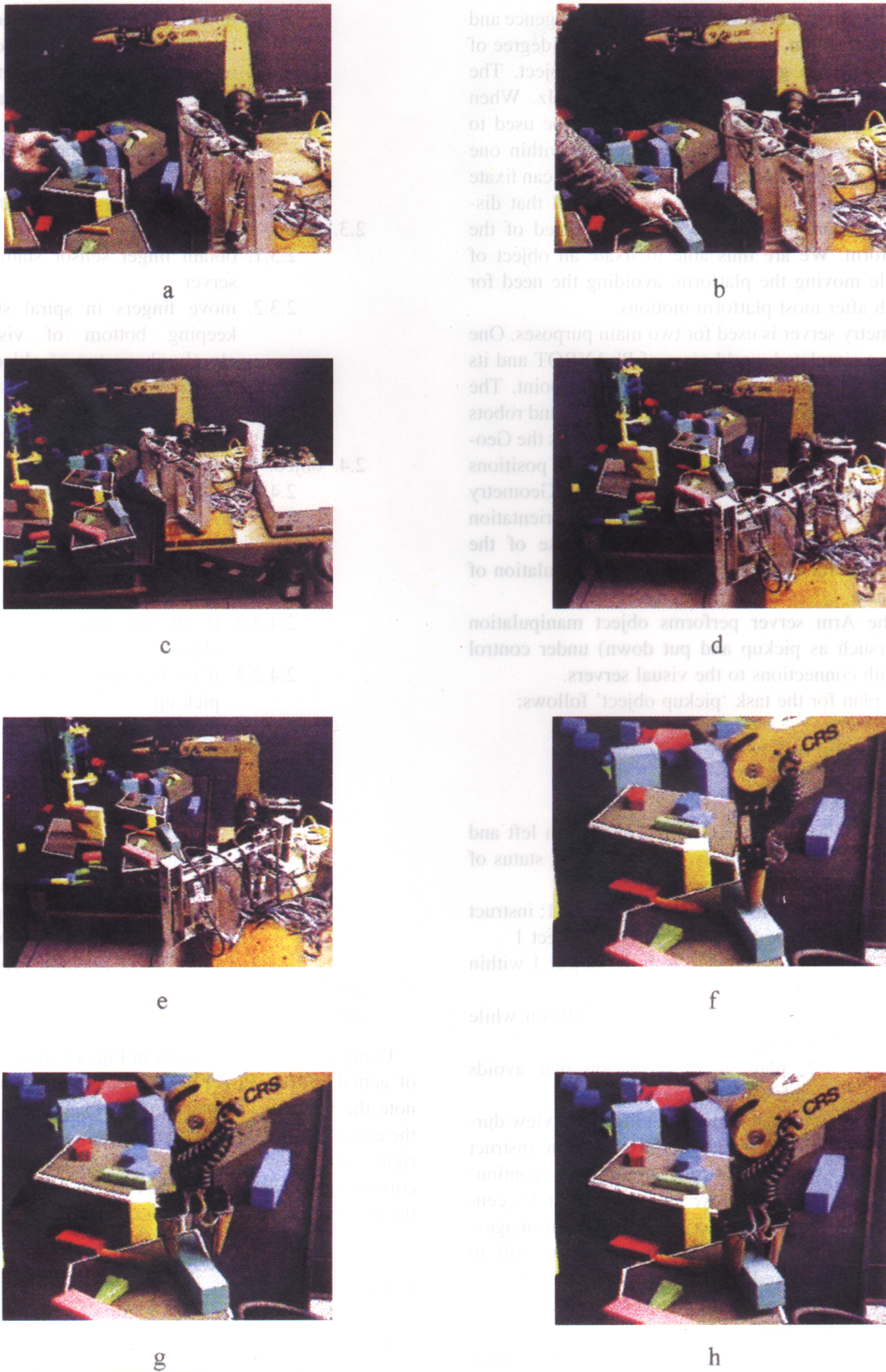
Fig. 13. Eight successive views of executing a 'pickup object' task. The correspondence of images to task steps is: (a) 1; (b) 1; (c) 2.1.1; (d) 2.1.3; (e) 2.2.1; (f) 2.2.4; (g) 2.4.1; (h) 2.6. Note that the object is placed in the field of view by a human, and may be placed anywhere in the camera's current field of view constrained by positions that are actually reachable by the robot, for this implementation.
