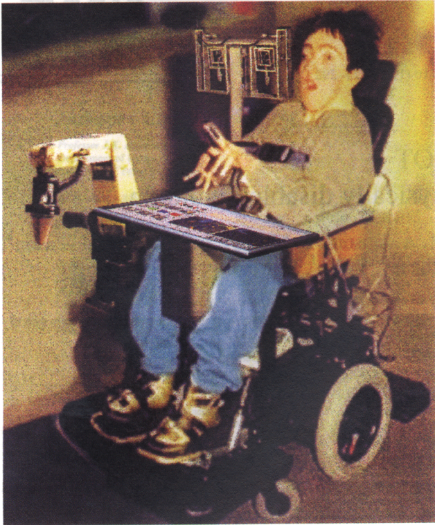
Fig. 1. Artist's conception of PLAYBOT (actual child in a wheelchair on which is superimposed PLAYBOT specific components, robot arm, user interface and TRISH stereo head).
