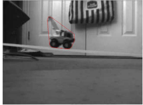
Fig. 3. This figure shows the convex hull of intensity constraints used to initialize an active contour around the tow truck. The red line is the active contour's starting point in the first frame.
