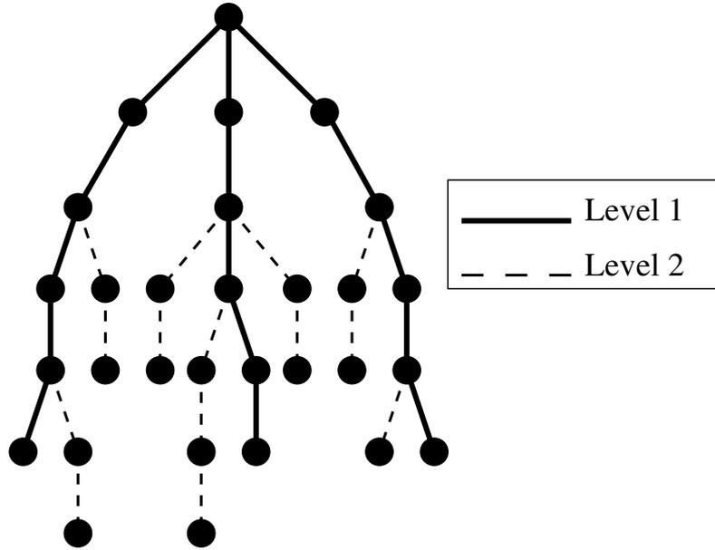
Fig. 8.8. Path partition of a tree
