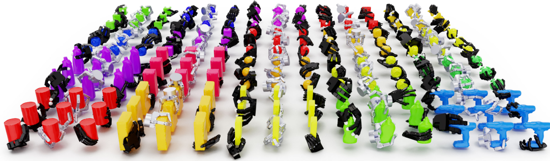
Fig. 1: The Grasp'D-1M dataset contains one million unique grasps, each with multi-modal visual inputs for training vision-based robotic grasping. We synthesize these grasps with a new differentiable grasping simulator, Fast-Grasp'D . Gradient information accelerates the grasp search, allowing us to search the full-DOF space (without eigengrasps) and simulate thousands of contacts to produce a dataset of contact-rich, stable grasps that can improve any learned grasping pipeline.
