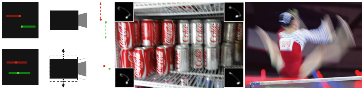
Motion Blur, Fig. 1 With motion blur, the amount of blur depends on the relative motion between the camera and the scene objects; it depends on the focal length and of the lens and the scene depth and motion trajectories. An example of
