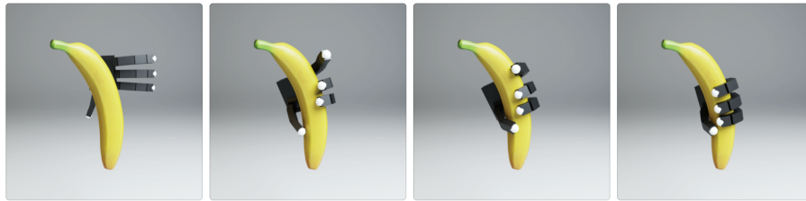
Fig. 2: Our method can synthesize grasps for both human and robotic hands, such as the four-finger Allegro hand in this figure. After hand initialization, we run gradient-based optimization to iteratively improve the grasp, in terms of stability and contact area. We include additional examples in Appendix B.
