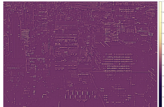
Result of applying the filter kernel to the input image by convolution – bright areas show strong response to this particular filter – so they resemble the feature it represents
