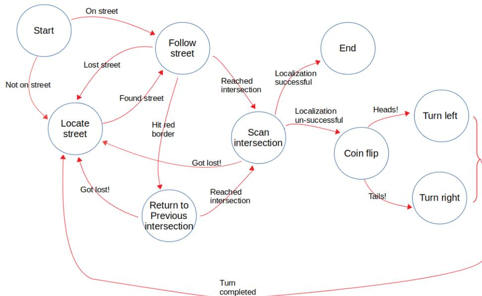
A few things are worth noting from the diagram. First, there is always a **start state** which takes care of any initialization required for the robot (in this case, setting up initial probabilities for each intersection, and figuring out if the robot is or is not on a street at the beginning of the process). There is also an **end state** which is reached once the robot has achieved its (or one of its) goal(s).
