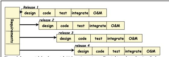
Figure 4: Incremental development. Initial requirements are allocated to a planned series of releases.
