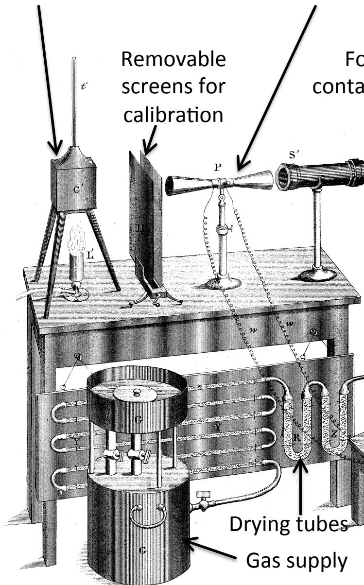
Thermo-electric pile to compare temperatures
