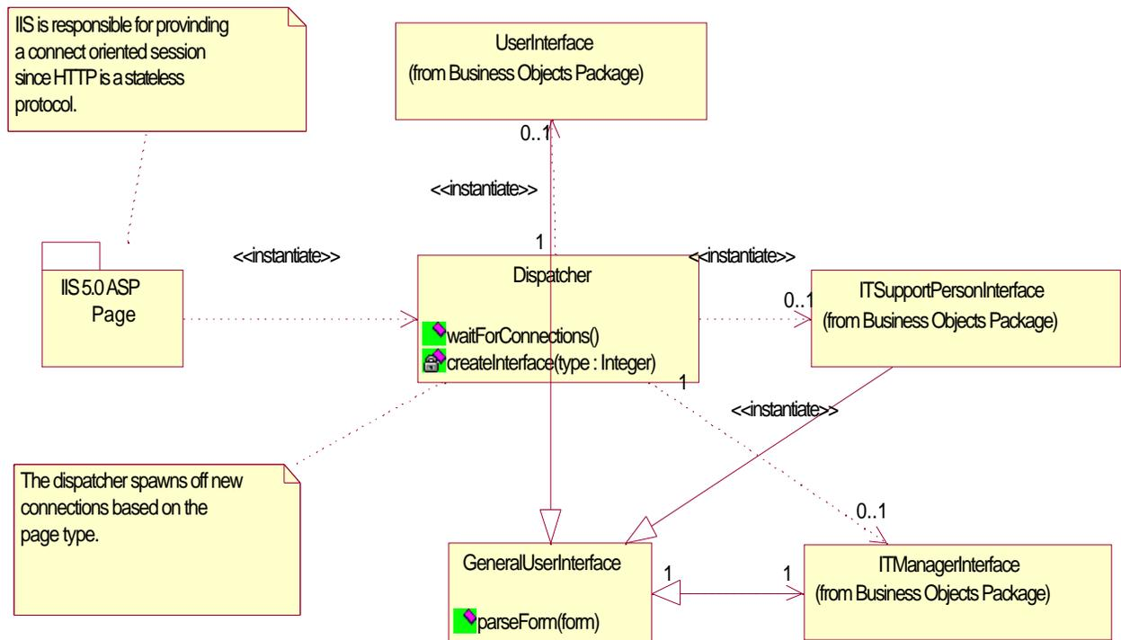
**Figure 5 User Interface class diagram**
