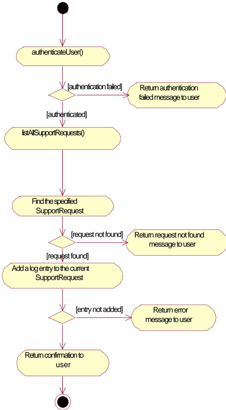
Figure 9 addEntryLogToRequest() Diagram
