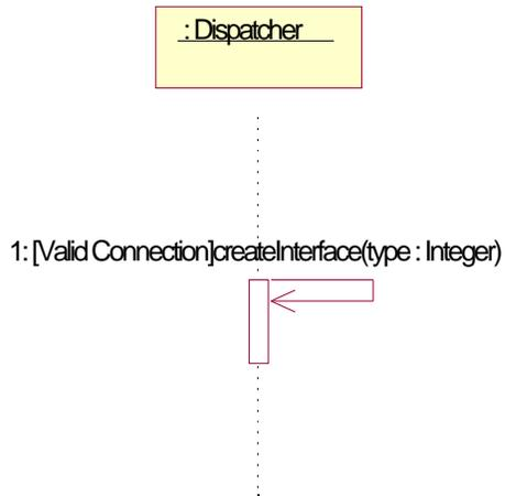
**Figure 17** `waitForConnections()` Sequence Diagram
