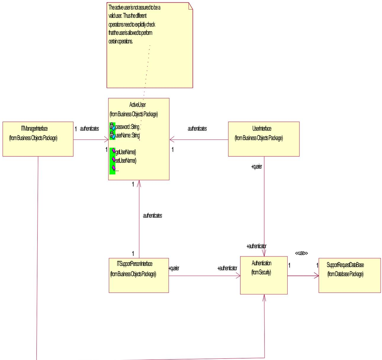
**Figure 3 Security Class Diagram**
