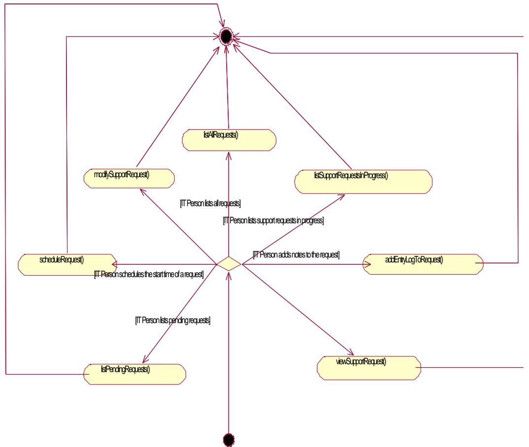
Figure 8 ChooseAction() State Diagram
