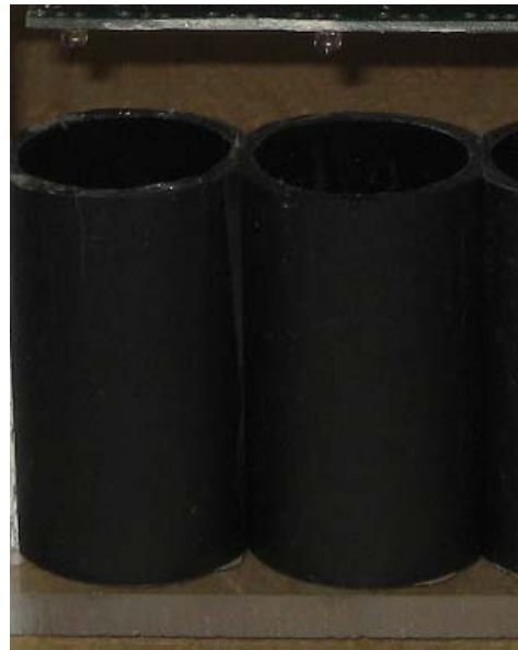
FIGURE 10-5, INFRARED LED AND TUBE FOR ISOLATION
