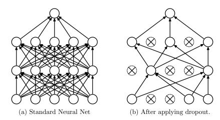
Figure 1: Dropout Neural Net Model. **Left**: A standard neural net with 2 hidden layers. **Right**: An example of a thinned net produced by applying dropout to the network on the left. Crossed units have been dropped.
