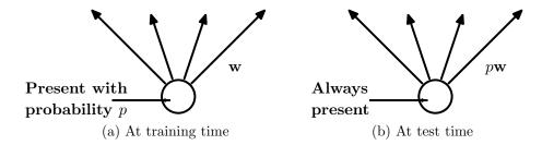
Figure 2: **Left**: A unit at training time that is present with probability p and is connected to units in the next layer with weights  $\mathbf{w}$ . **Right**: At test time, the unit is always present and the weights are multiplied by p. The output at test time is same as the expected output at training time.
