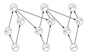
The output unit should compute the XOR of the current input and previous output:
