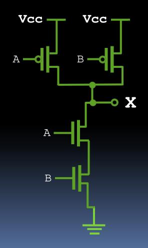
Remember: transistors that look like are activated when the gate input is high, whereas transistors that look like are activated when the gate input is low.
