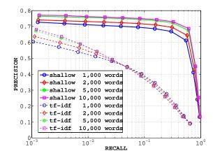
Figure 6. Precision-recall curves for the 20 Newsgroups dataset comparing the performance of tf-idf versus a one-layer shallow model with 200 code units for varying sizes of the word dictionary (from 1000 to 10000 words).
