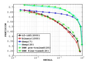
Figure 7. Precision-recall curves comparing compact representations vs. high-dimensional binary representations. Compact representations can achieve better performance using less memory and CPU time.
