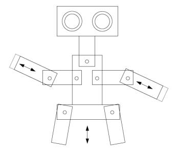
It has seven rotational joints, depicted with small circles; each has one rotational degree of freedom. The outer limbs of each arm scale non-uniformly outward along the given arrows, providing two more degrees of freedom. The entire character moves up and down as indicated by the arrow near the base, providing one translational degree of freedom.
