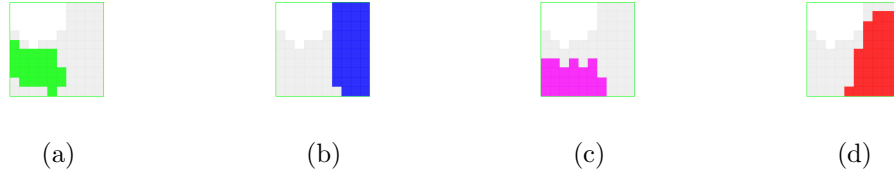
Figure 8.4: (a)-(d) The 4 regions of the decomposition of real visibility data collected in a 2m by 2m space, sampled at 20 cm intervals.
