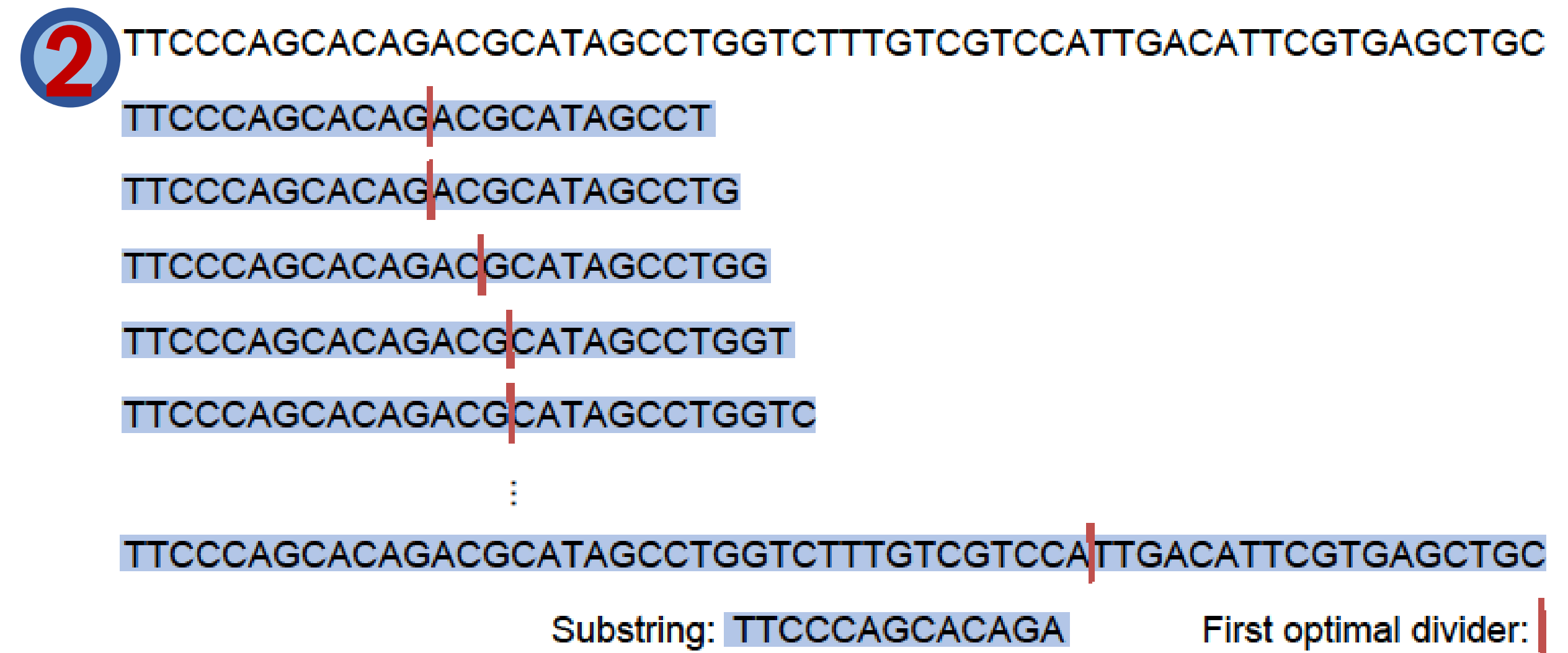
Fig 2: In OSS, only substrings that starts from the beginning of R is examined. Among all substrings, the first optimal divider, P , of a shorter substring comes earlier than a longer substring, therefore, "cascading" the optimal dividers
