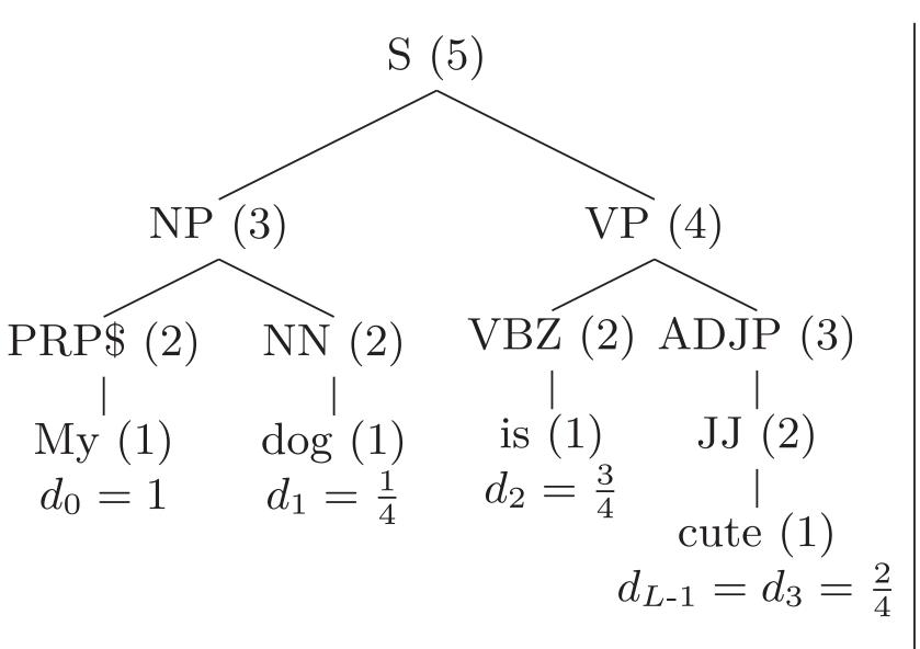
An RH distance calculation example. The heights of nodes (h) are in brackets.
