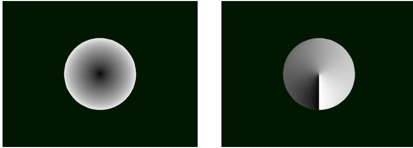
Figure 3.3: Spherical Coordinates for View Vector. The figure visualizes \phi values per pixel (left) and \theta values per pixel (right).
