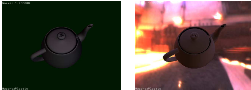
Figure 3.14: Magenta Plastic. The plastic material demonstrates the diffuse property of the BRDF data.
