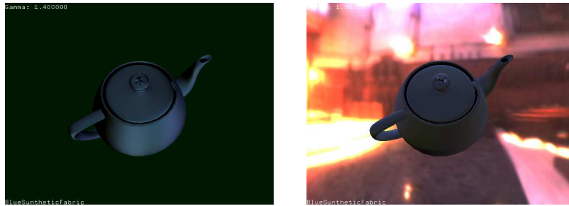
Figure 3.9: Blue Synthetic Fabric. A directional light vector illuminates the teapot from above (left), and a set of 128 lights determined by using the Median-Cut algorithm illuminates the teapot with the Grace Cathedral light probe (right).
