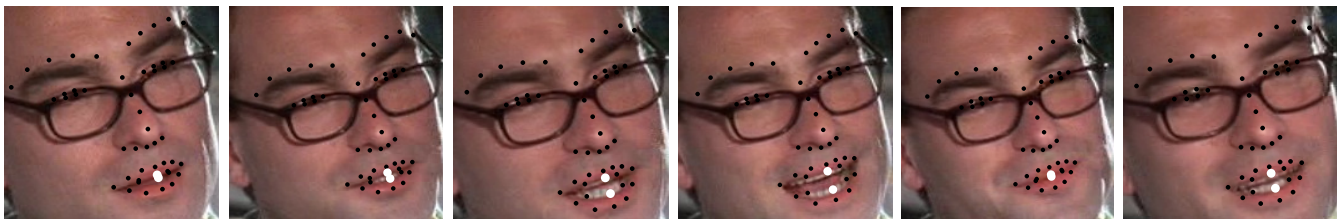
Fig. 2. SDM-based facial landmarks on faces from a track. The landmark points are presented in black, while the points used to measure the amount of mouth opening – upper lip lower center and lower lip upper center are marked in white.
