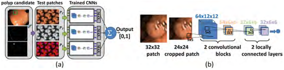
Fig. 5. (a) The test stage of the suggested score fusion framework. (b) Network layout used for training the deep convolution networks.
