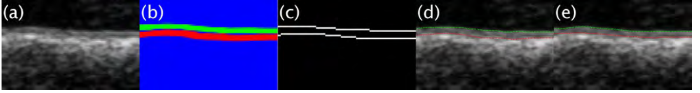
Fig. 8. The test stage of lumen-intima and media-adventitia interface segmentation. (a) A test region of interest. (b) The corresponding confidence map generated by the convolutional neural network. The green and red colors indicate the likelihood of a lumen-intima interface and media-adventitia interface, respectively. (c) The thick probability band around each interface is thinned by selecting the largest probability for each interface in each column. (d) The step-like boundaries are smoothed using 2 open snakes. (e) Interface segmentation from the ground truth.
