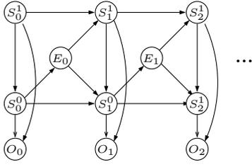
Figure 2: DBN encoding of a 2-level hierarchical HMM.
