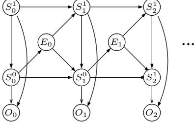
Figure 2: DBN encoding of a 2-level hierarchical HMM.
