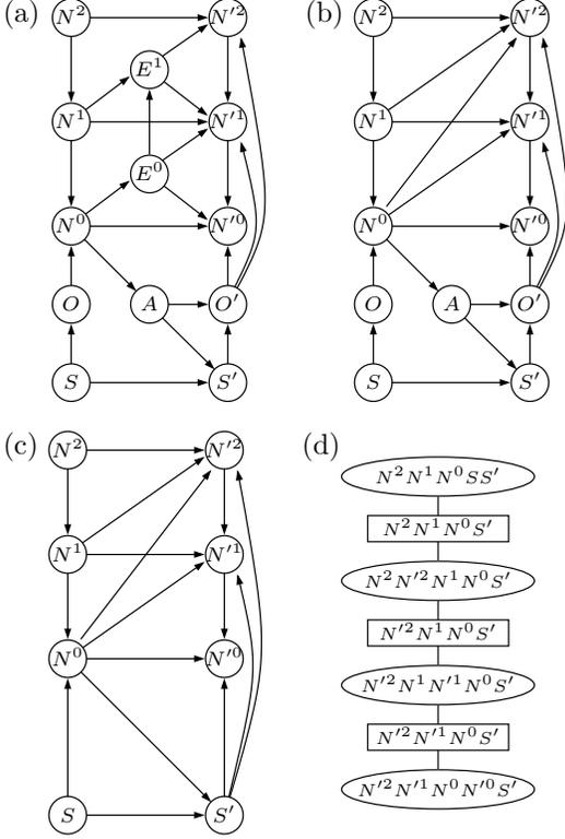
Figure 3: (a) Two slices of the DBN encoding the hierarchical POMDP controller. (b) A version where exit variables are eliminated. (c) Variables  $O$  and  $A$  are eliminated. (d) The corresponding junction tree (or rather chain) for inference.
