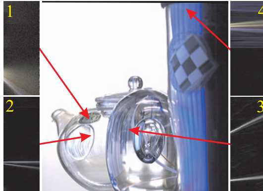
Figure 2: Center, back to front : a teapot made of thin glass about 2mm-thick; a solid crystal ornament with an internal air bubble; a mug with a 2mm-thick enclosure made of clear plastic and an opaque interior cavity made of a purple specular material (see Figure 6, bottom right for another view). Sidebars : Scatter traces for the four pixels indicated by arrows. These pixels receive light (1) by direct reflection at an opaque point; (2) by direct reflection and by internal reflection at the back-surface of the thin teapot wall; (3) by direct reflection and by a secondary internal reflection; and (4) by direct reflection, internal reflection at the back-surface of the clear enclosure, and internal reflection off the purple interior. Note the distinct “traces” associated with each propagation mode.
