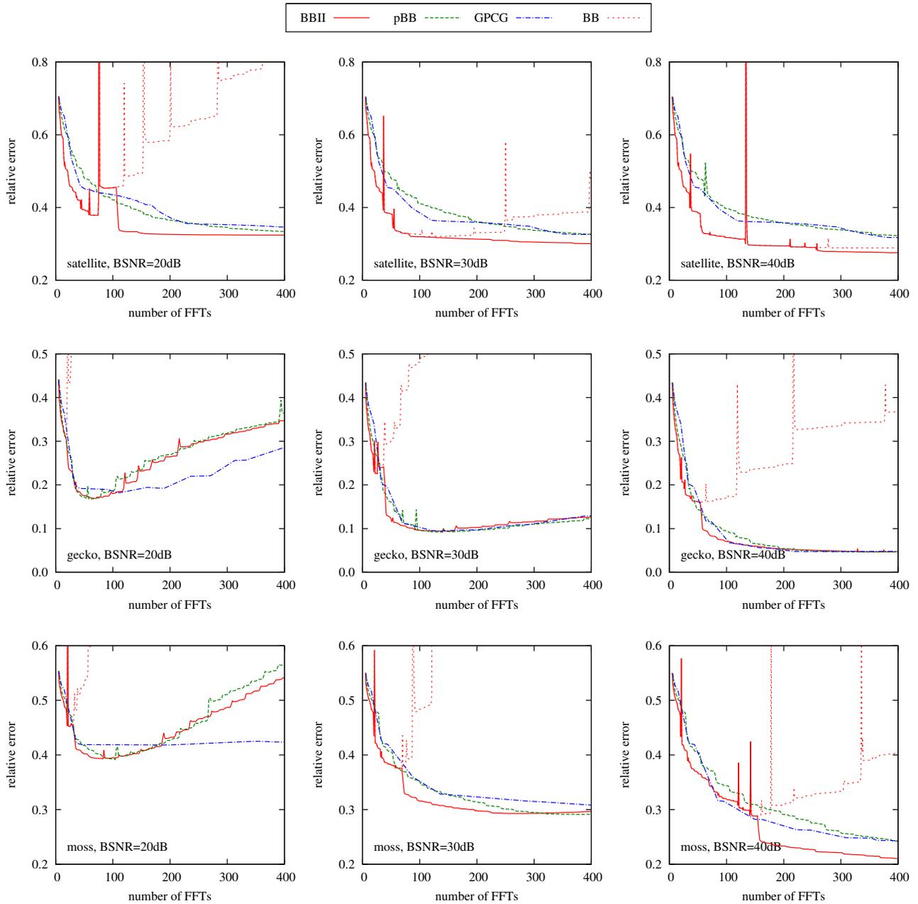
Figure 4. Relative error plotted against the number of FFTs for BBII, BB, pBB, and GPCG. Test images are, from top to bottom, satellite, gecko, and Irish moss. Blurred signal to noise ratios are, from left to right, 20dB, 30dB, and 40dB.
