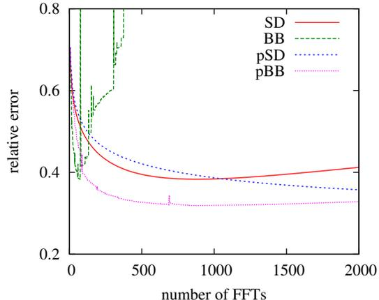
Figure 1. Relative restoration error plotted against the number of FFTs for the steepest descent, Barzilai-Borwein, projected steepest descent, and projected Barzilai-Borwein methods applied to the deblurring of the satellite image with BSNR = 20dB.
