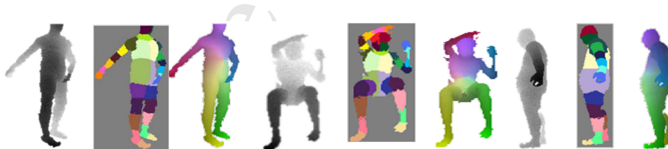
Fig. 7 Training data used to train the PARTS and MSIG forests. We show here three example training images in triplets. For every triplet, we show left to right : (1) the synthetic depth image, (2) the body PARTS output label and (3) the MSIG output. Because the synthetic images have been generated using the model, every pixel can be annotated with the
