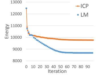
Figure 2b: **Levenberg-Marquardt (LM) vs. ICP.** A standard (ICP) like algorithm that alternates between discrete updates of  $\mathcal{U}$  and continuous optimization of all other parameters (ICP) converges extremely slowly, whereas simultaneous optimization of all parameters (LM) converges rapidly.
