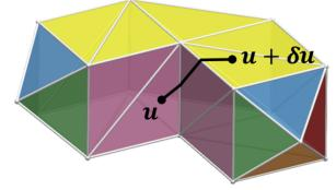
Figure 3: Illustration of mesh walking to apply Levenberg-Marquardt update  $\delta \mathbf{u}$ .
