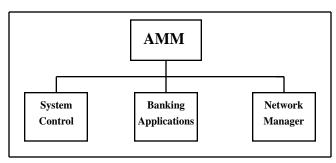
**Banking Applications Subsystem** includes use cases for banking transactions and their inputs and outputs.
