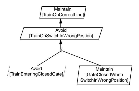
**Goal** Avoid[TrainOnSwitchInWrongPostion] **Definition** When a train is on a switch, the switch should be in the direction of travel of the train
