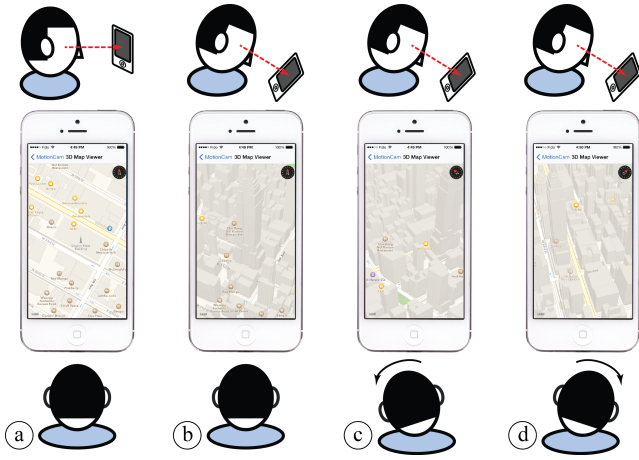
Figure 5: 3D map viewer: (a) normal 2D viewing, (b) rotating the phone to enter the 3D view mode, and (c)(d) moving the head to glimpse left or right side of the 3D buildings.
