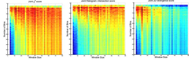
Figure 2. Joint score for the  $\chi^2$  (left), histogram intersection (centre), and JD-divergence (right) similarity measures for different window sizes and number of histogram bins. Blue indicates low scores, red indicates high scores.
