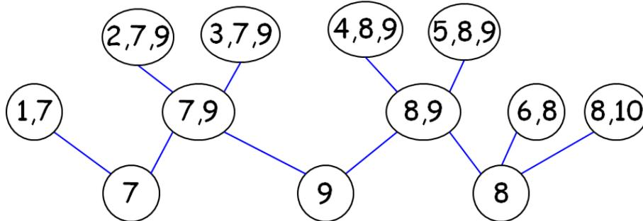
Here the maximal cliques  $M_j$  are the leaves, and their intersections form the intermediate vertices. Note the vertex labelled (9) is a subclique many of the leaves, but it is only a maximal subset of the vertices labelled (7,9) and (8,9). Therefore, by the above definition, there are only the two edges  $((9), (7,9))$ , and  $((9), (8,9))$  with the vertex (9) as an endpoint.
