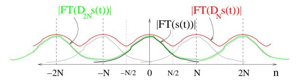
Aliasing destroys information about the original continuous signal whenever there are significant nonzero coefficients,  $a_n$ , for any frequency larger than the Nyquist frequency  $\omega_{N/2} = \pi$  (i.e. after sampling we only have access to  $\hat{a}_n$  not  $a_n$ ).
