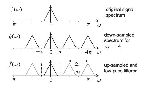
Here the replicas can be isolated by an ideal low-pass filter (the dotted pass-band), so the original signal can be perfectly reconstructed.
