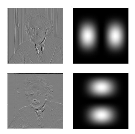
**Top Row:** Convolution of Al with a horizontal derivative filter, along with the filter's Fourier spectrum. The 2D separable filter is composed of a vertical smoothing filter (i.e.,  $\frac{1}{4}(1,2,1)$ ) and a first-order central difference (i.e.,  $\frac{1}{2}(-1,0,1)$ ) horizontally.
