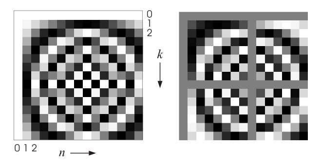
**Left:** This shows the real part of the inverse DFT matrix,  $\cos(2\pi nk/16)$ , with frequencies  $\omega_k = 2\pi k/16$  for  $0 \le k \le 15$  from top to bottom. The spatial variable n increases from 0 to 15. The first row and column are filled with ones.
