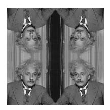
The DCT requires only one quadrant in this response. (We show all four for comparison purposes.) Note the responses for horizontal and vertical gratings have been significantly reduced.
