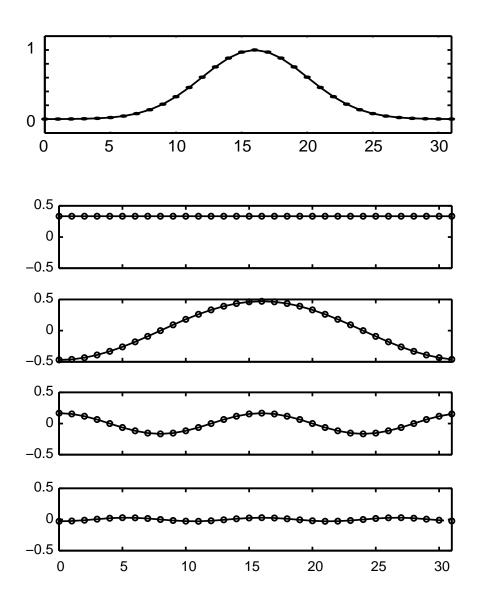
A Gaussian signal is shown on top with 32 samples. The first 4 terms of its Fourier decomposition are shown below, with frequencies  $2\pi k/N$  for  $0 \le k \le 3$ . The amplitudes of these first 4 Fourier coefficients are 0.3333, 0.47, 0.166, and 0.029.
