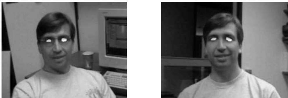
Figure 1: Results of eigen-eye pair detector for the first and last frames. White regions indicate the detected eyes.
