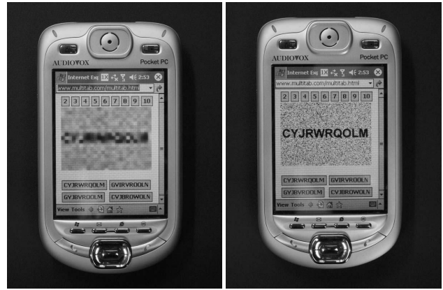
Figure 1: Snapshot of the PDA with the multi-tab interface that allows users to select an arbitrary fidelity level. The left and right snapshots show the same image at low and high fidelity, respectively.
