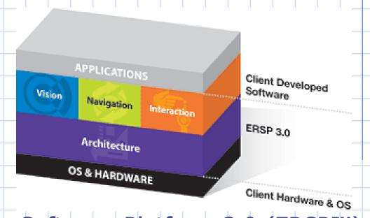
The Evolution Robotics Software Platform 3.0 (ERSP™) is a comprehensive development platform with four primary areas of functionality: vision, obstacle avoidance, interaction, and architecture. ERSP 3.0 includes library APIs, developer tools, and applications to aid you in the robot development process and allow you to move to higher-level programming quickly.
