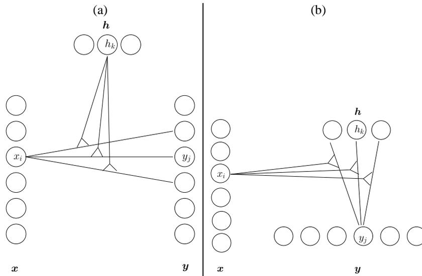
Figure 1: Two views of the basic model. (a) Gated regression: Hidden units can add slices  $W_{..k}$  into a blend of linear transformations. (b) Modulated filters: Input units gate a set of basis functions that learn to reconstruct the output.
