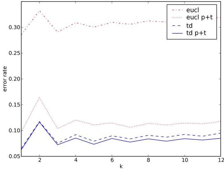
Figure 9: Error rates using k-nearest neighbors. The model induced distance is compared with the Euclidean distance for two different training sets. Adding affine transformed digits to the training set helps the Euclidean distance a lot, but it is of very little help to the learned distance because the model can learn about transformations from the basic training set.
